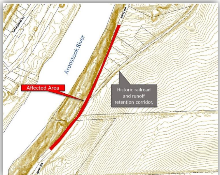
Figure 2: Area topography (2' contours) showing general drainage slopes toward the affected areas. Note the area of steep slopes between the road and the river.
