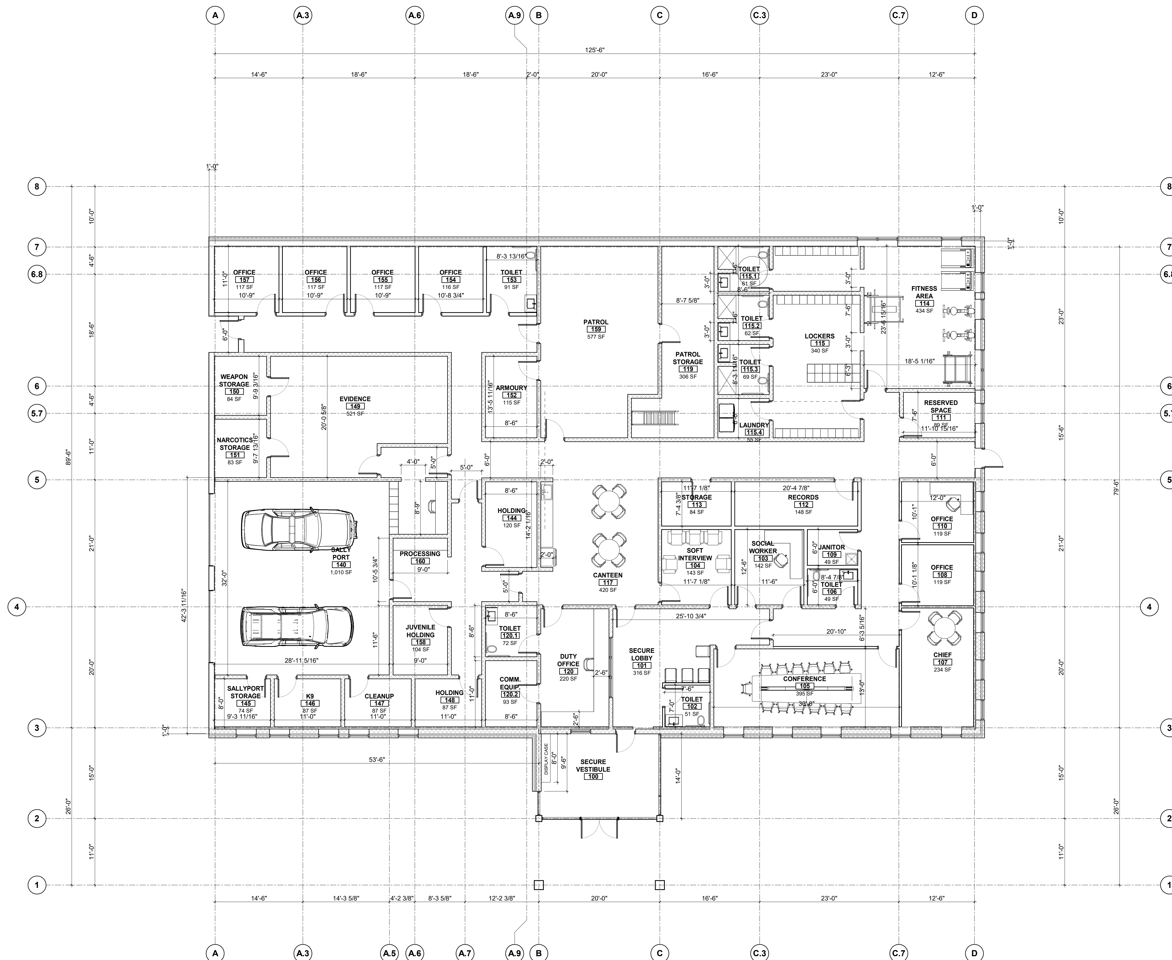
1 FIRST FLOOR DIMENSION PLAN 1/8" = 1'-0"
