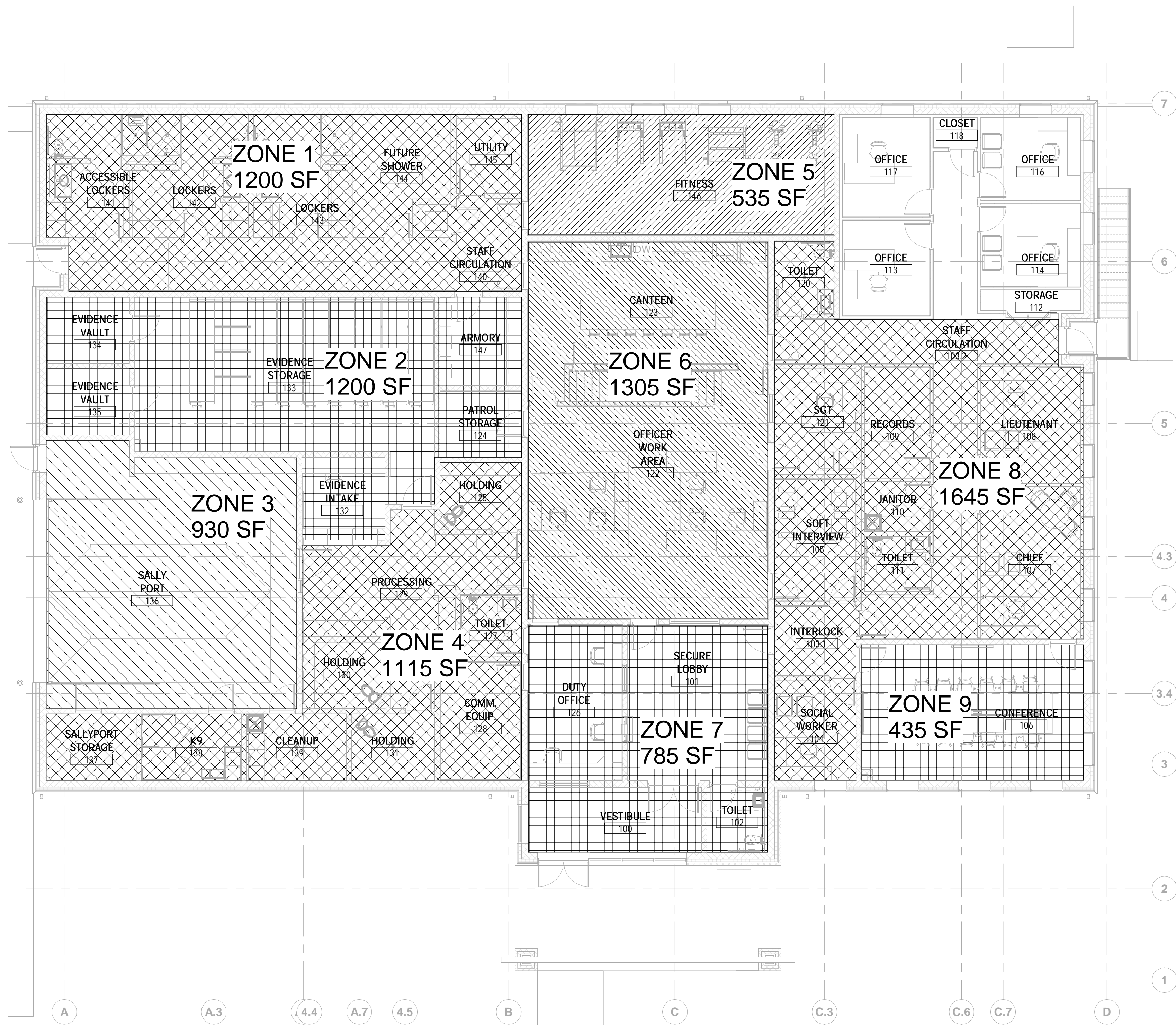
RADIANT FLOOR ZONING PLAN SCALE: 1/8" = 1'-0"
