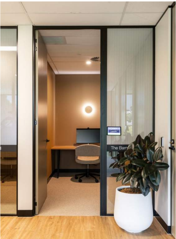
TELEHEALTH ROOMS Frosted glass doors to allow light to pass through but provide privacy. Acoustical materials on walls for additional audible privacy, play with color and pattern to make space feel warm and not clinical.
